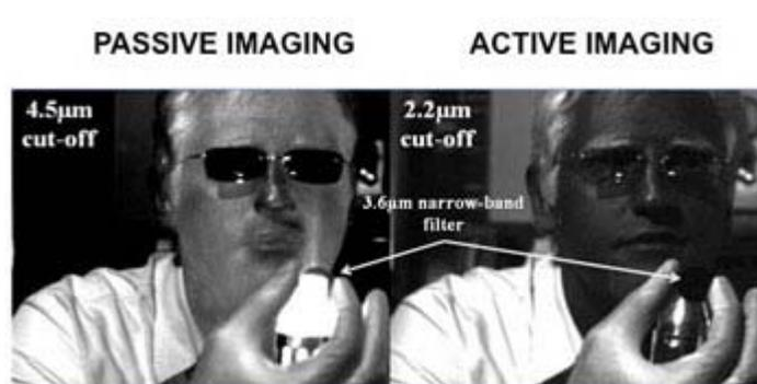
A Center for Quantum Devices researcher holds a heater and a narrow-band filter centered at  $3.6\mu\text{m}$ . The heater can be seen when imaged with the band-pass detectors sensitive up to  $4.5\mu\text{m}$  (left), but not in the ones with shorter detection wavelengths up to  $2.2\mu\text{m}$  (right).
